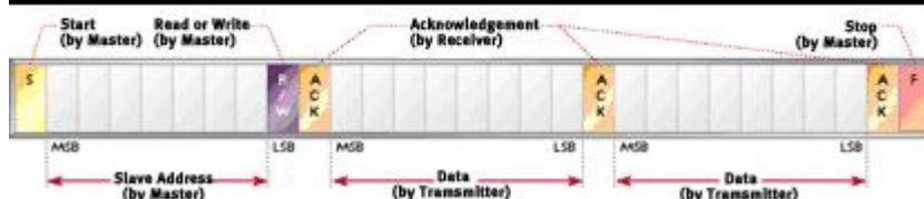
Figure 2: I 2 C communication
